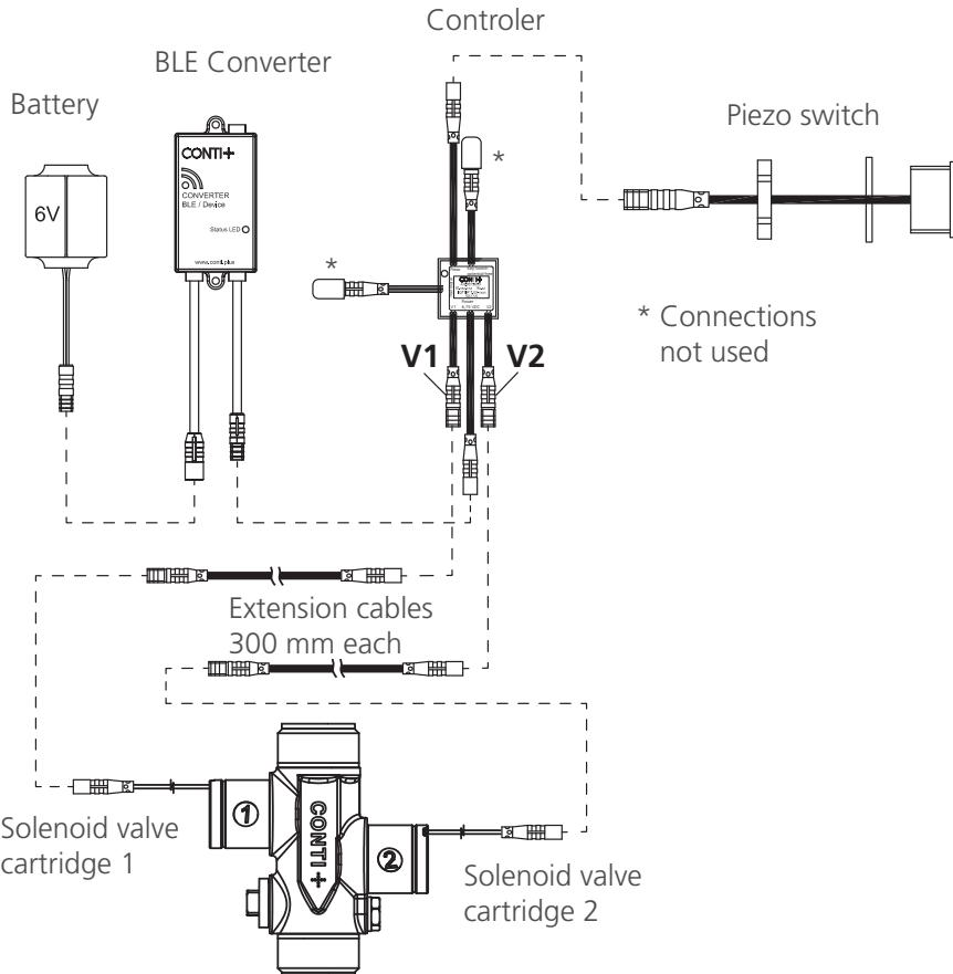
! To save battery capacity, the BLE Converter automatically switches to sleep mode when not in use. In sleep mode, settings via the ServiceAPP are not possible. To exit sleep mode, the piezo switch must be pressed 8x (4x water flow). After 2 minutes of inactivity, the BLE Converter switches back to sleep mode.
