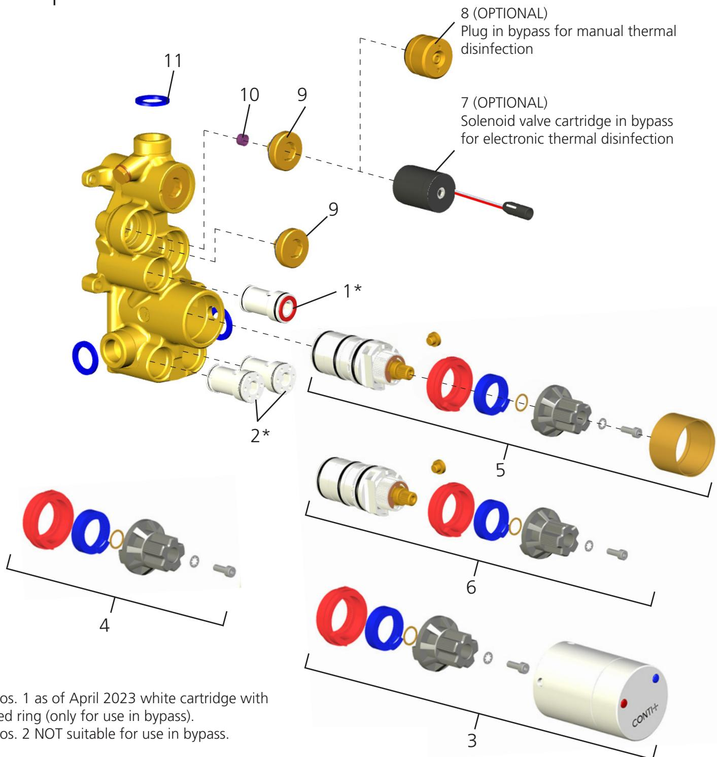
\* Pos. 1 as of April 2023 white cartridge with red ring (only for use in bypass).
