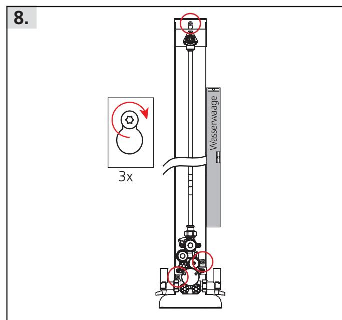
Screw down the rear panel, observing the perpendicular alignment.
