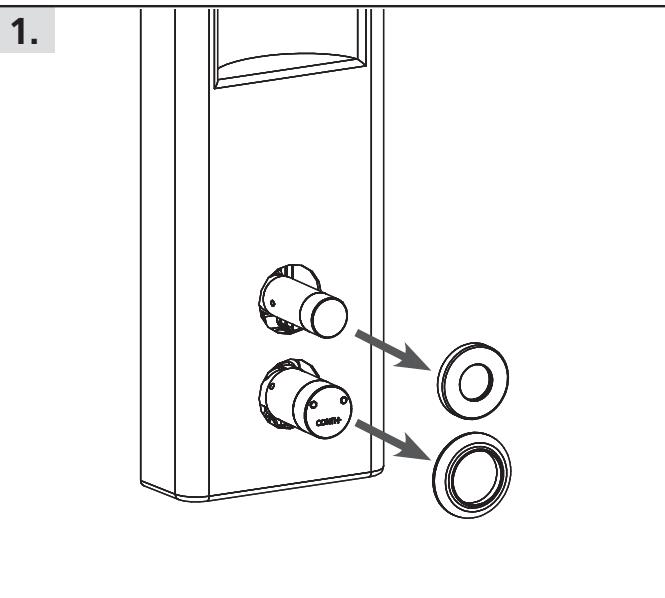
Pull off the rosette including the O-ring from the trigger and the rosette including the deflector ring from the thermostat handle.
