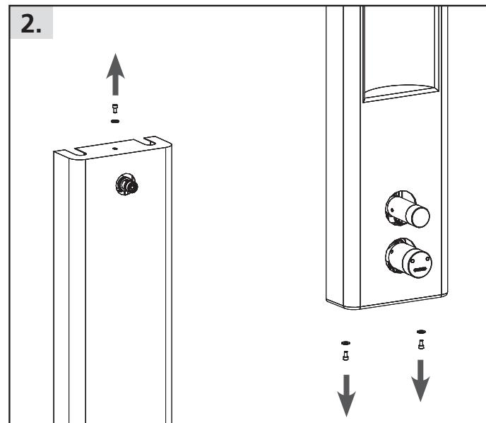
Remove the hood screws at the top and bottom and remove the hood.
