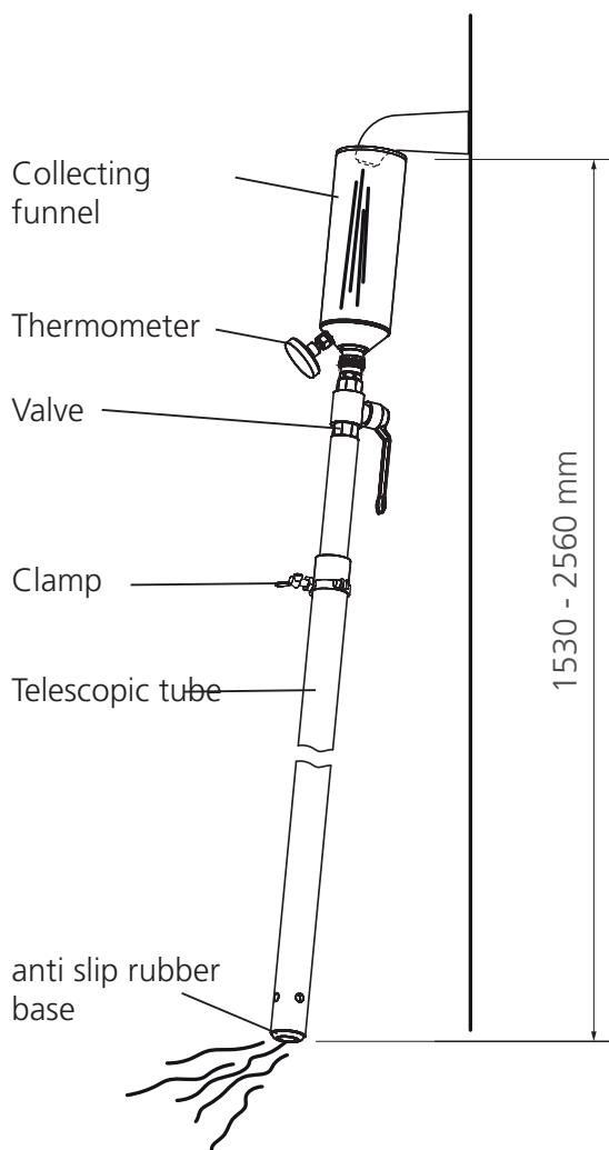
Clamp the service pipe between the shower head and the floor using the adjustable length of the pipe.
