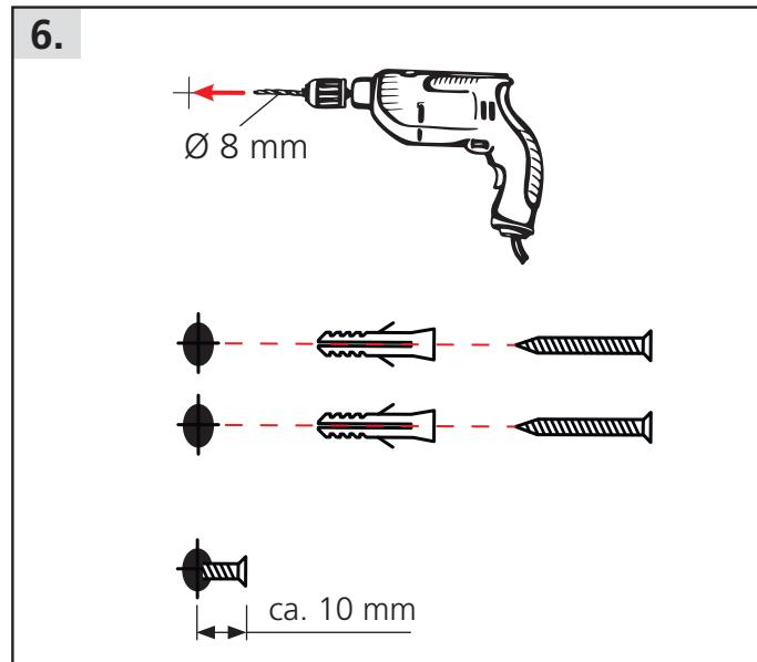
Drill holes, insert dowels and screw in screws (TORX SW25). Allow screw heads to protrude by about 10 mm.
