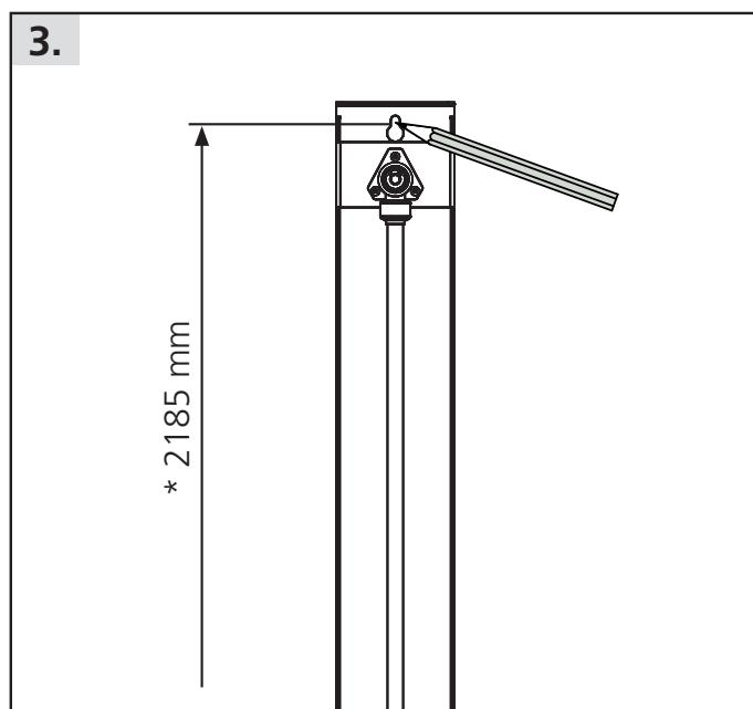
\* For installation height recommendation 2200 mm from top edge of finished tiled floor.
