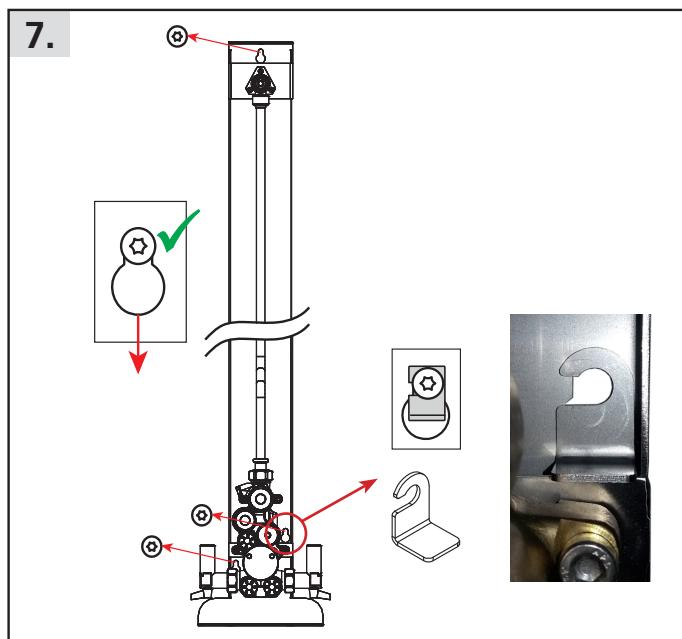
Hang the rear panel and attach the securing bracket to the lower, right attachment as shown.
