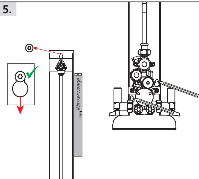
Hang the back panel on top, align with spirit level and mark bottom holes.
