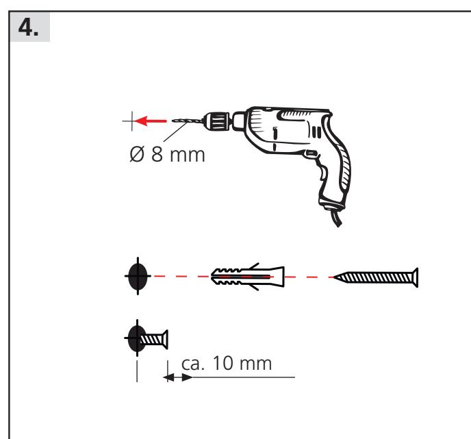
Drill a hole, insert the dowel and screw in the screw (TORX SW25). Allow the screw head to protrude by approx. 10 mm protrude.
