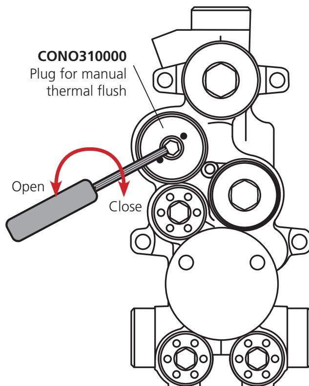
To perform a manual thermal flush, insert a hexagonal wrench (SW3) into the bypass plug and open the valve
